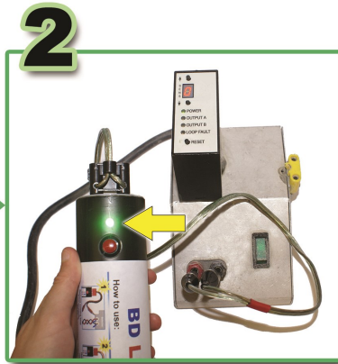
Hook E-Z Detector Checker in replace of loop.
