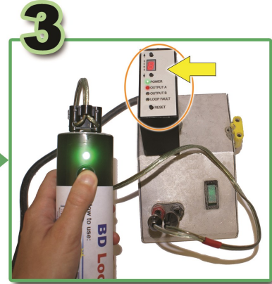
Reset the detector and press the red button on the E-Z Detector Checker to simulate a car trip.
