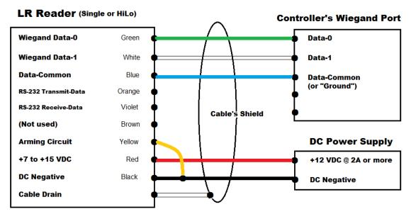
Figure 2 Wiring for LR-3000 Installation
