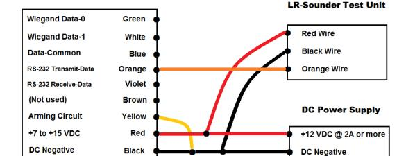
Figure 3 Wiring for quick test
