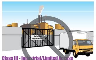
**Vehicular Gate Operator**A vehicular gate operator (or system) intended for use in an industrial location or building such as a factory or location of
