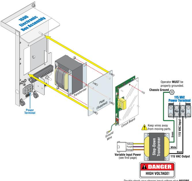
Double check your chosen input voltage plug **BEFORE** applying power to the step-down transformer. Failure to choose the **CORRECT** input voltage plug for your desired input voltage **WILL damage** operator and **VOID** warranty.
