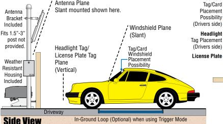
**Tags/Card Placement on Cars:** It should be placed on the side of the car (headlight/windshield) closest to where the antenna is located. The tags/card needs to be placed in **visual sight** of antenna or antenna can **NOT** read tags/card. **Never** place tags/card in a position that will block the drivers vision.
