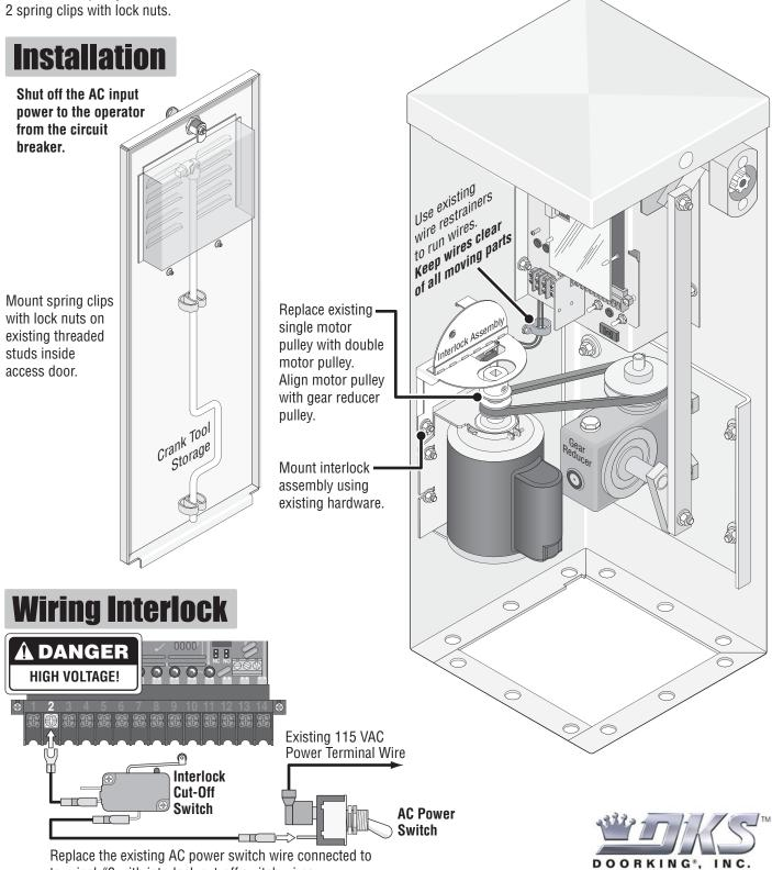
terminal #2 with interlock cut-off switch wires.
