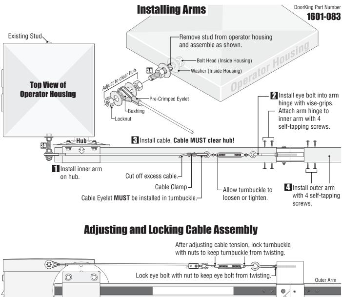
Inner Arm  $\bigcirc$  $\bigcirc$ 0 Rotate arm up and down. Adjust cable tension with turnbuckle to level outer arm. Make sure that cable assembly is not binding **Side View of** or twisting and everything moves freely. **Operator Housing** Important: Do not adjust cable too tight or it will bind.
