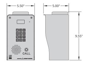
Hole pattern on back for pedestal mounting is spaced at 3.063" with pilot holes for alternate mounting at 2.5".
