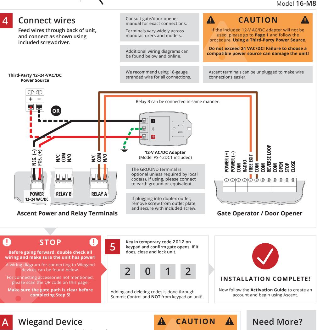
Feed wires through back of unit, and connect as shown using included screwdriver.
