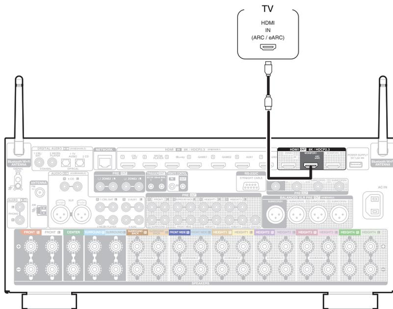
\* For 4K TVs we recommend using an HDMI cable labeled “High Speed” and “with Ethernet”.
