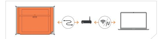
Connect your Mr Beam to your router via a network cable (Ethernet). The network socket is located on the rear below the USB ports.
