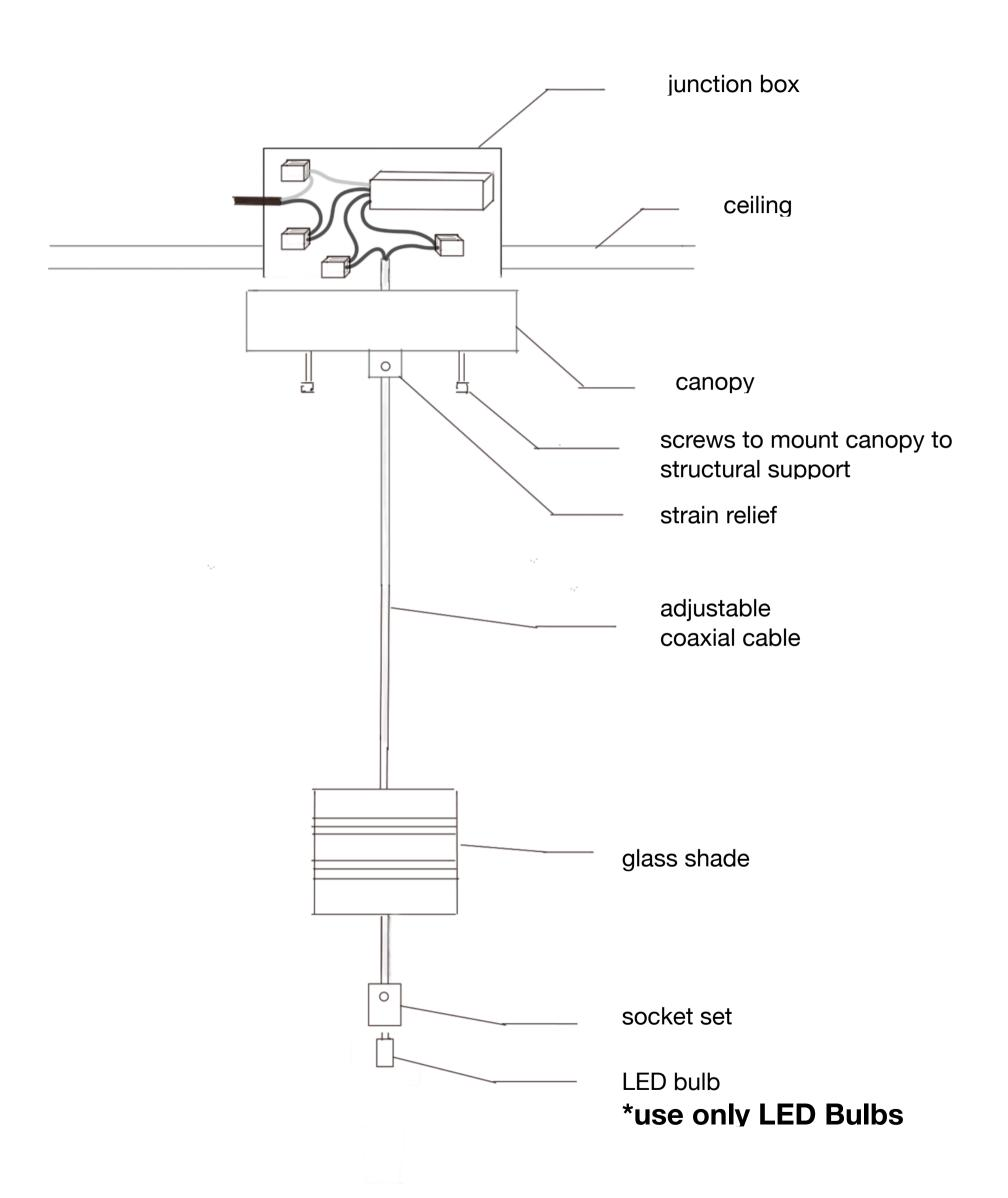
Carefully unspool coaxial cable to avoid kinks in the line.
