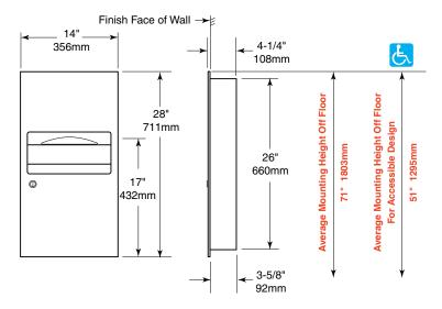
Rough Wall Opening 12-1/2" (318mm) Wide 26-1/2" (673mm) High 3-3/4" (95mm) minimum recessed depth
