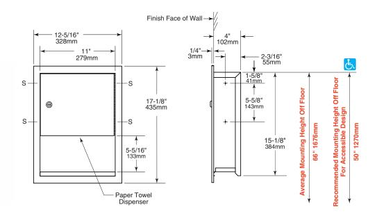
**Rough Wall Opening** 11-1/4" (286mm) wide 15-5/8" (397mm) high 4" (102mm) minimum recessed depth
