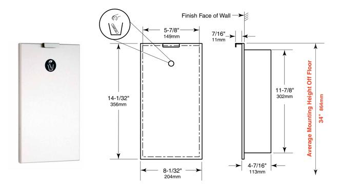
Rough Wall Opening 6" (152mm) Wide 12" (3051mm) High 4" (102mm) minimum recessed depth
