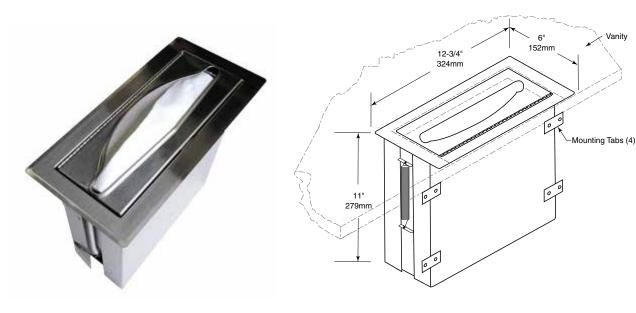
Rough Countertop Cutout 11-1/4" (286mm) Wide 4-1/2" (114mm) High 3/4" to 1-1/2" (19 to 38mm) mounting thickness 17" (430 mm) minimum clearance below mounting surface
