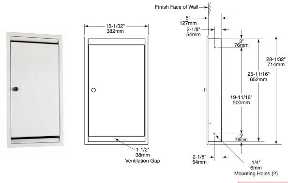
Rough Wall Opening 13-1/2" (343mm) Wide 26-1/2" (673mm) High 4-3/4" (121mm) minimum recessed depth
