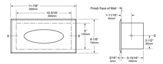
**Rough Wall Opening** 10-3/4" (275mm) wide 5-1/4" (135mm) high 4" (102mm) minimum recessed depth
