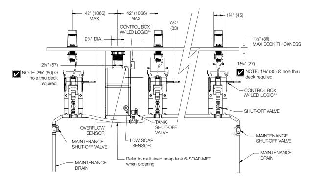
\*\* NOTE: Battery pack or AC adaptor required. AC power source required to be within 54" (1371) of the control box.
