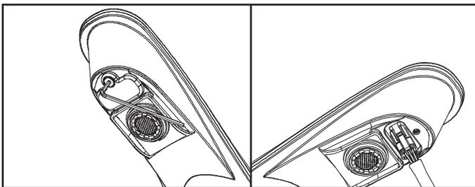
Loosening screw will cause sensor assembly to back out of spout body. It may be necessary to push cable from connector end to aid in sensor assembly removal. Firmly press into pocket and tighten screw. Sensor connector may need to be turned horizontally when first inserting into the spout.
