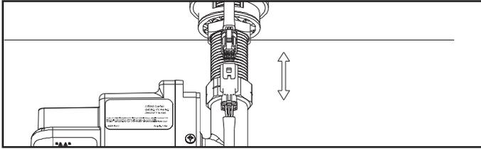
Use supplied 3/32" hex wrench to loosen set screw. Screw will retract into the base to eliminate loss. Using the same hex wrench, depress the ball detent to release spout from base.
