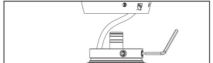
Align spout so that the ball detent is between the 2 holes. Press down and turn clockwise. Use hex wrench to back set screw out to secure spout
