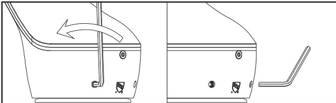
To reinstall faucet, first drop sensor cable of new spout through the front of the base. Lower spout onto base inserting base nipple into spout port.
