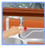
Grip connector with one hand and with free hand, push down outer ring.
