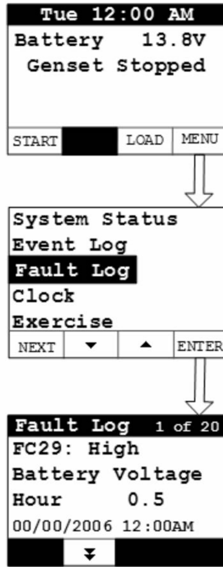
FIGURE 13. FAULT LOG SCREEN
