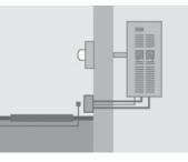
The GenReady load center is installed with the EZ Transfer operator. All fuel and electrical lines (contractor supplied) are installed to the planned generator site along with the generator pad (if required). The home is completely wired and ready for the addition of a generator in the future.
