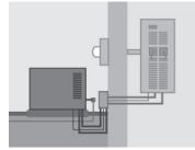
Everything included in the GenReady Advanced level is installed along with an automatic standby generator. The home's selected circuits will be backed up by generator power whenever the utility is lost.
