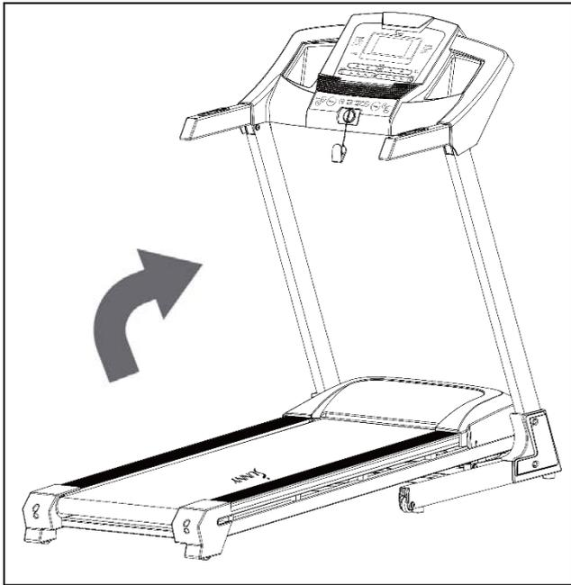
**NOTE:** Please make sure the incline is at ZERO when folding and unfolding.
