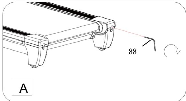
2. If the **Running Belt (No. 50)** drifts to the left, turn the left adjusting bolt  $\frac{1}{4}$  turn **clockwise**, then turn the right adjusting bolt  $\frac{1}{4}$  turn **counter-clockwise**. If the **Running Belt (No. 50)** does not move, repeat this step until it centers. Refer to image B.
