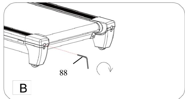
3. Over time, the **Running Belt (No. 50)** will loosen. To tighten the **Running Belt (No. 50)**, turn both the left & right side adjusting bolts one full turn **clockwise**. Check the tension of the **Running Belt (No. 50)**. Continue this process until **Running Belt (No. 50)** is at the correct tension. Make sure to adjust both sides equally to ensure even alignment. Refer to image C.
