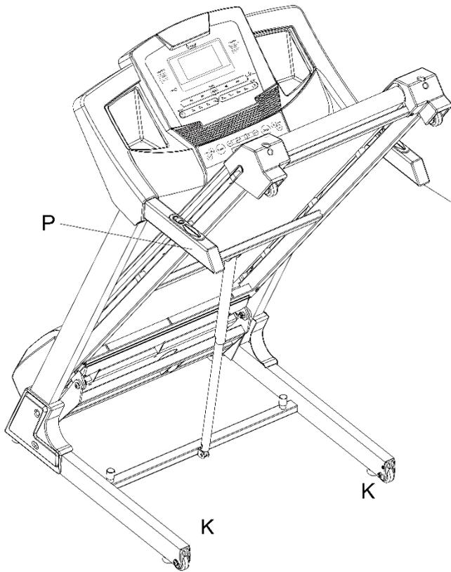
Before attempting to move the treadmill, make sure that it has been properly folded. Then, unplug the power cord.
