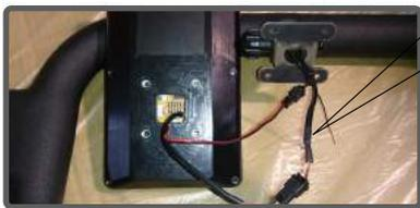
※ Connect RPM and resistance wires.
