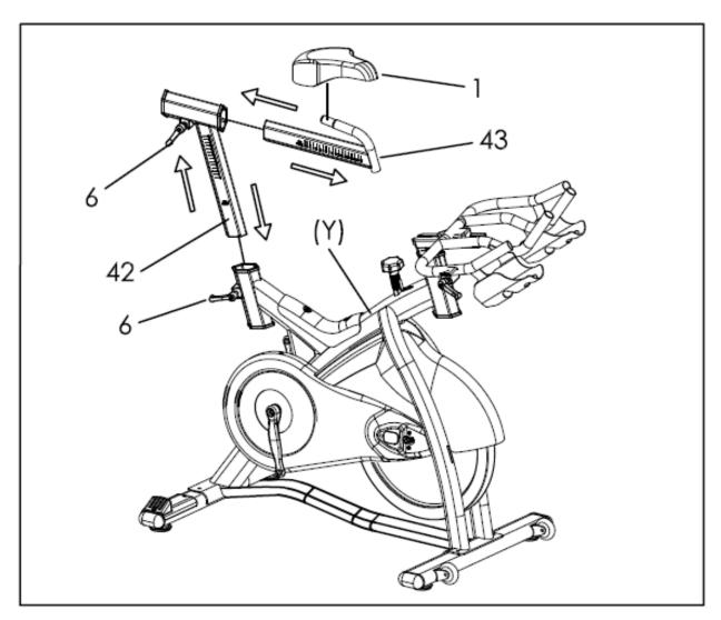
Insert the Seat Post (42) into the seat tube located on the Main Frame (Y).
