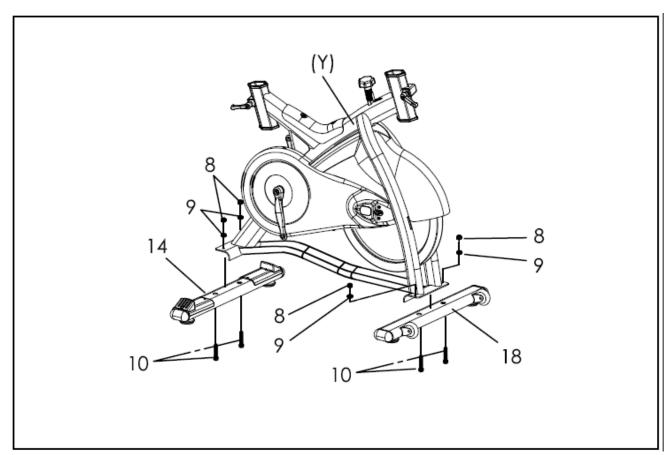
Attach the **Front Stabilizer (18)** and the **Rear Stabilizer (14)** to the Main Frame (Y) using 4 **Bolts (10)**, 4 **Washers (9)** and 4 **Nuts (8)**. Tighten and secure using spanner wrench.
