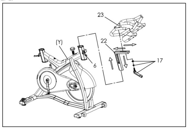
Loosen adjustment L-Shaped Knob 1 (6) on main frame handlebar tube to remove insert protect cap, then insert the Handlebar Post (22) into the handlebar tube of the Main Frame (Y). Move Handlebar Post (22) to the desired height. Tighten the L-Shaped Knob 1 (6) to secure the Handlebar Post (22) into position.
