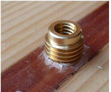
The insert nut will be re installed with the screwdriver slot on the bottom
