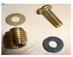
Vent parts. ¼-20 brass screw with a notch cut in it. The brass Insert nut has self tapping threads.
