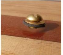
The vent screw doesn't have to be completely removed or even raised all the way. The slot in the screw just has to be near the top
