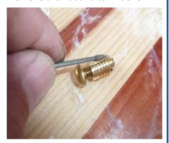
Coat the threads with 5 min. epoxy. Don't over do it here or you could get excess epoxy in the threads.
