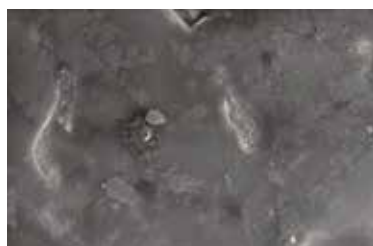
Porcelain surface before being etched
