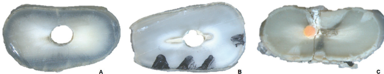
Figure III. Representative images of the failure pattern analysis by digital stereomicroscopy after the bond strength test, after the use of different intracanal medication removal techniques of Bio-C Temp (Angelus) and Ultra Cal XS (Ultradent). (A) Dentin adhesive failure; (B) Mixed adhesive failure; and (C) Cohesive failure.
