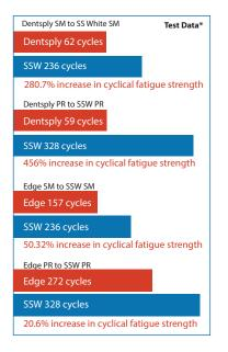
Cyclic fatigue is the leading cause of file separation. EXACTFlowH<sup>™</sup> rotary files offer a remarkable leap forward in resistance to cyclic fatigue.
