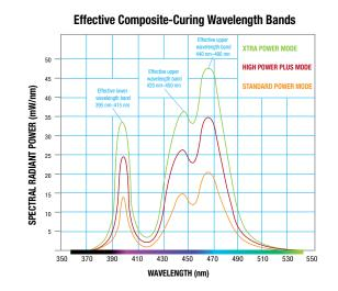
All VALO LED curing lights use a custom, multiwavelength light-emitting diode (LED) for pro-ducing high-intensity light at 385-515 nm, which is capable of polymerizing all light-cured den-tal materials. Every member of the VALO curing light family also offers three curing modes to accommodate your preferences.
