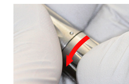
After use, twist the handle to unlock
