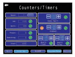
Digital display tracks production and makes it easy to manage process elements like Index Dwell, Preheat Mode, Flash Duration, and Flash Delay.
