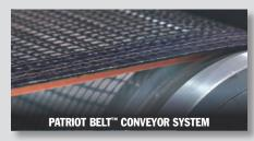
Patriot Belt<sup>™</sup> with the SureTrak<sup>™</sup> roller system features a heatresistant, Teflon®-coated fiberglass belt with a red flexible bead stitched along one edge that rides in grooves machined into the large anodized aluminum rollers, providing the most precise belt tracking available (U.S. Patents Pending: SN 15194035 & 15265538)
