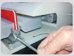
Insert the retaining pin and release the clamping mechanism by pressing either button
