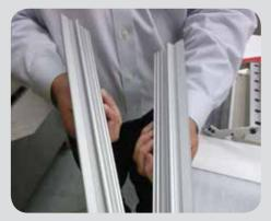
Hold a bar in each hand with the interlocking sides facing each other
