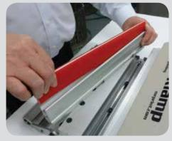
Seat the squeegee blade in the opening between the two sides and place the set between the Qwik-Klamp's jaws
