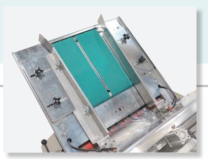
Infeed chute with belt-driven system delivers shirts quickly and accurately to the bag
