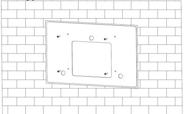
2. Align the holes of the beauty plate with the holes on the wall. Tighten the screws into the holes to secure the beauty plate.
