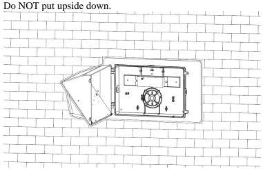
Install wall pack fixture (14" housing) according to the footprint of beauty plate.
