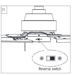
Setting the reverse switch in the left hand side will result in downward airflow and setting the switch in the right hand side will result in upward airflow. **Note:** Reverse switch must be set either way completely. If the reverse switch is set in the middle position, fan will not operate.
