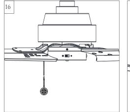
Install fan pull chain to preassembled pull chain on fan. Pull chain provided.
