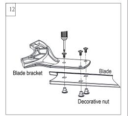
Install blade bracket with blade by 3 blade screws and decorative nuts provided. Tighten screws securely. Repeat this process for remaining blades.
