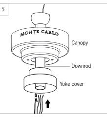
Place downrod over canopy and yoke cover. Thread lead wires and safety cable from motor assembly through downrod.
