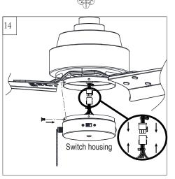
Remove set screws from top cover of switch housing. Keep screws. Connect the plug from fan to the plug from switch housing, aligning the claps and make sure plugs connected securely. Install witch housing, aligning the holes on switch housing with screw holes on top cover and reinstall the set screws.
