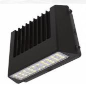
Our Full Cutoff Wall Pack has zero up light and a type IV forward distribution that produces a pattern of light meant for mounting on the sides of buildings and walls. Along with its built-in photocell, it has multiple wattages and CCT's to choose from. The housing is a powder-coated die-cast aluminum and very easy to install.
