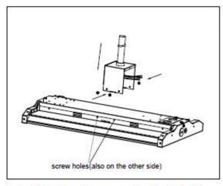
Install the two side-covers of the bracket with screws to hide the wires.
