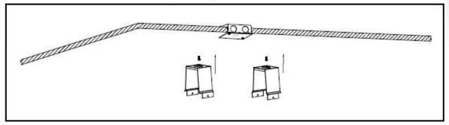
2. Fix the fixture to the bracket with adequate screws.
