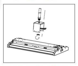
Make wiring connections refer to General Wiring Diagram. The bridged wires must be UL listed and wrapped with flexible protective conduit.
