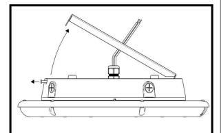
1. Loosen the two screws holding down the Quick Mount Bracket (QMB) until the QMB is able to hinge freely. Do not remove these screws.
