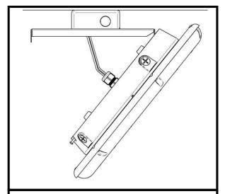
4. Hook the fixture to the QMB by sliding the fixture over the T-Flanges, reversing the motion performed in Step 2. Gently move the fixture through its full range of motion to ensure it is hanging securely.
