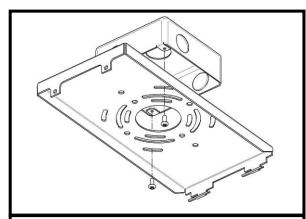
3. Mount the QMB to the junction box or ceiling using appropriate hardware (supplied by others). The QMB must be installed with a minimum of two screws, but four is recommended.
