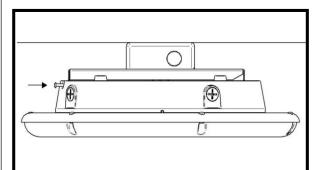
6. Tighten the two screws indicated above until they sit flush to the casting.
