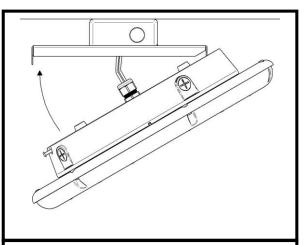
5. Complete all wiring of the fixture. Feed all wiring Connections through the center hole in the QMB into the junction box. Swing the fixture up until the holes in the QMB align with the two screws loosened in Step 1.
