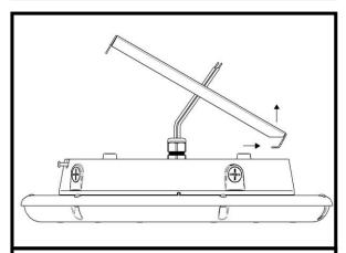
2. Remove the QMB from the fixture by sliding the QMB towards the back of the fixture and lifting up.
