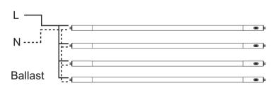
Step 2. For single ended use, lamp is compatible with non-shunted lamp holder ONLY.
