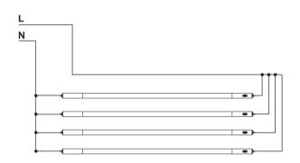
Step 1. Cut all wires connected to the existing ballast, remove the ballast.
