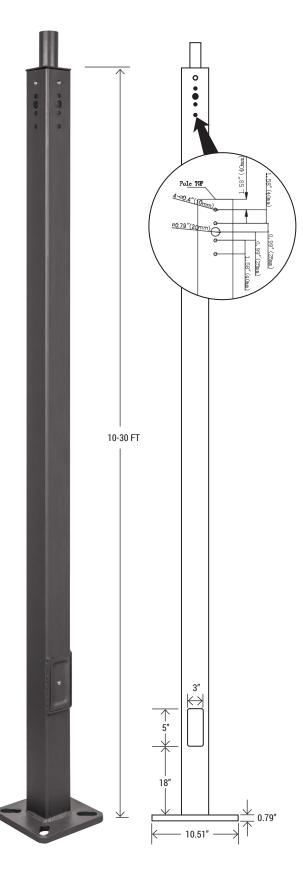
The WSD LED INC Series Straight Square Steel poles are built from high strength steel tube and are available side drilled for arm mounted area lighting luminaires or with tenon mounts for flood and post top luminaires. Typical area lighting applications include retail centers, industrial parks, schools and universities, public transit and airports, office buildings and medical facilities. Mounting heights of 10 to 30 feet can be used based on selected luminaire application.
