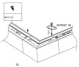
Use the M4x12 to lock the connection plate with fixture on back
