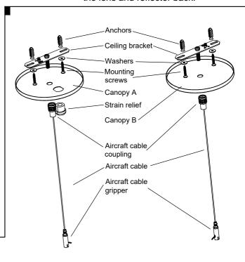
How to disassemble the Surface mount kit
