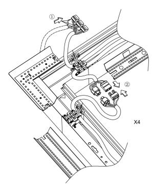
First Step: Take off the lens and reflector to connect the corner fitting and fixture together
