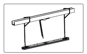
5.Reattatch the luminous part to the housing to complete the installation.
