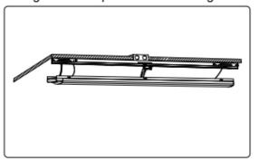
Fix the baffle onto the back of the fixture with screws.
