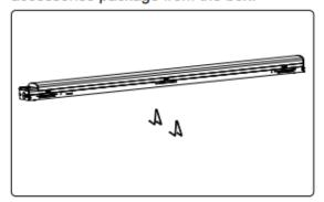
3.Attach chain to the V-hooks to hang the luminaire.
