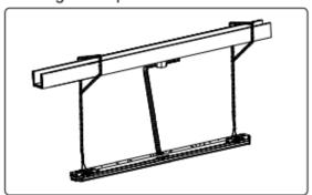
2.Connect the V-hook to back of the fixture body.
