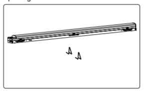
3.Attach the V-hooks to the fixture body to hang the luminaire.
