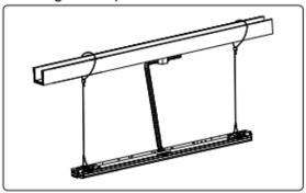
2.Attach V-hooks to the cable.
