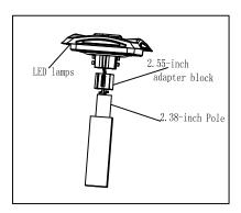
1). When the light pole is 2.38 inches, a 2.5-inch adapter shall be installed on the light fixture. Assemble as shown in the picture and tight the bolts on both sides of the lamps
