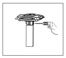
2) Lock the screws on both sides of the lamps, fix the lamps on the pole.
