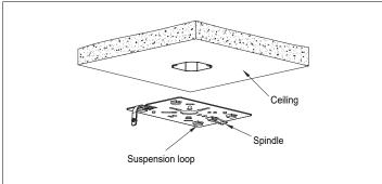
3. Connect the clip on the fixture to the spindle of the mounting plate to make sure the fixture will not slip and fall.connect the line voltage to the wires coming out from the fixture following the wiring diagram. Push the pressing plate into the suspension loop on the mounting plate.
