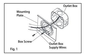
2. Pull wall box wires through center hole of mounting plate. Secure mounting plate to wall using screws so that the fixture mounting points are aligned vertically. (See Fig. 1)
