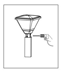
2.Lock the screws on both sides of the lamps, fix the lamps on the pole.
