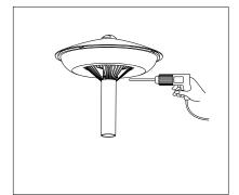
2) Lock the screws on both sides of the lamps, fix the lamps on the pole.
