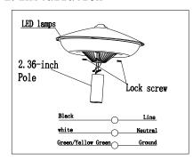
1). Connect the AC wire of the lamp as shown in the picture, then insert the lamp into the 2.36-inch pole.
