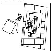
4) . After hanging the lamp on the mounting plate and tightening the screws, And put a waterproof glue seal between the bottom cover and the wall to prevent water from entering the lamp.
